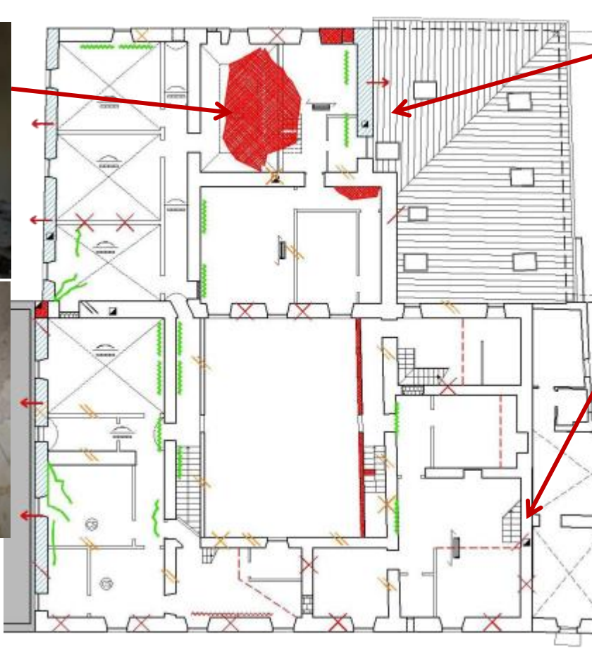
COLLAPSE OF THIN VAULTS
